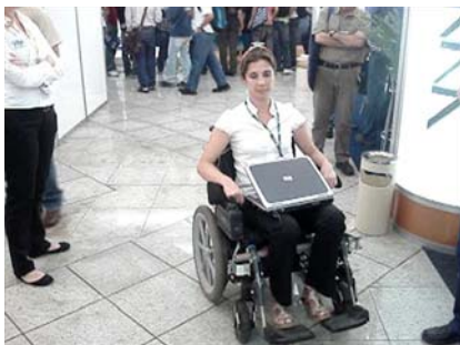
Fig. 6. Robotic wheelchair commanded by head movements (captured by accelerometer).
