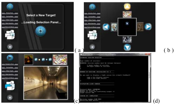
Fig. 4. Main windows of NEVRAROS Display Interface. (a) Primary module, which also load graphic elements such as mini map of the overall environment. (b) Selection module. Upper arrow is blinking for stimulating patient, and central cursor is moving for reaching desired destination. (c) Navigation module. While mobile device is reaching selected destination, a video stream is presented to user, as well as an intuitive indication of path selected (the room where the target resides is highlighted) and the overall progress of the path (little arrows on top indicate percentage of path already crossed). (d) Supervisor module, for tuning interface's parameters up.
