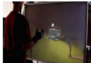
Fig. 8. The I-AUV is teleoperated by the user by means of special VR hardware, including immersive 3D vision and a virtual joystick controlled with data gloves.
