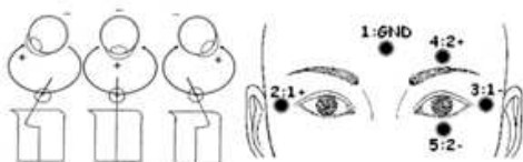
Fig. 3. Ocular dipole (right part). Position of the electrodes on the face (left part). 1: ground electrode, 2 and 3 for horizontal movement, 4 and 5 for vertical.
