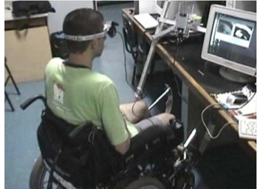
Fig. 11. Robotic wheelchair commanded by eye movements.
