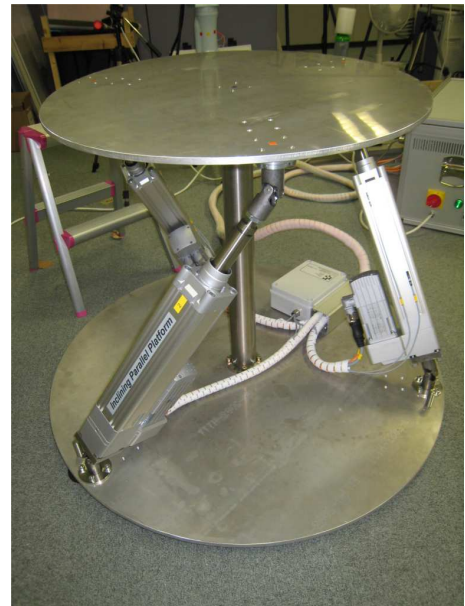
Fig. 6. Inclining parallel platform that can rotate around all three axes. The diameter of the platform is 0.7m and is able to carry an adult human.
