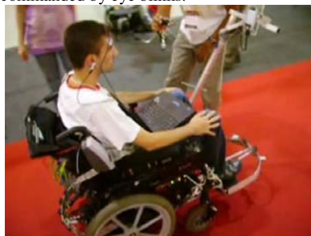
Fig. 3. Robotic wheelchair commanded by eye blinks.
