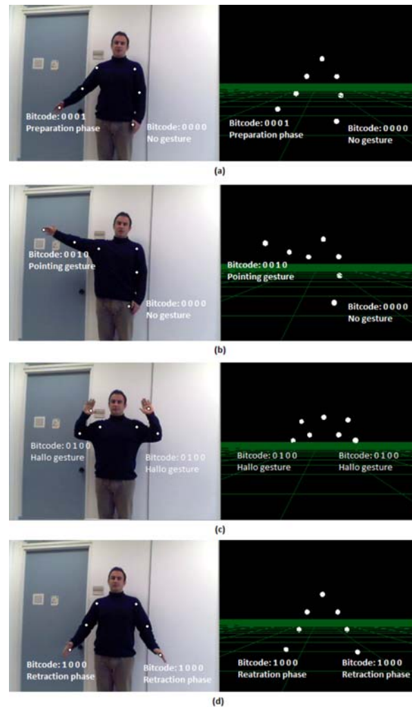
Fig. 6. Recognition and classification of gestures performed by one or both hands simultaneously. The left image depicts a 2D view from one camera of the stereo pair, while the right image shows the 3D representation (of the left image). The output of the classifier has been superimposed on the images for the sake of clarity. (a)The right arm prepares to perform a gesture. (b)The right hand performs a “pointing” gesture. (c)Both hands perform a “hello” gesture. (d)Both hands retract from the stroke phase.
