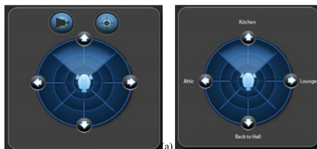
Fig. 1. (a) controlling a mobile device with six high-level commands: four directional arrows for direction decision, and two movements buttons for starting and stopping movement; (b) controlling a mobile device with four high-level destination commands: three select new destinations, one for going back to last destination.
